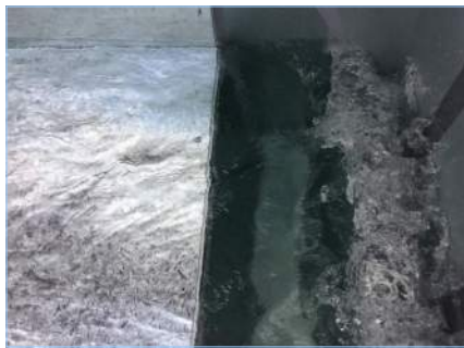
DB 600-1, Q = 16 l/s (box gutter slope - 1 in 200)
