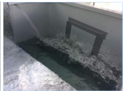
DB 600-1, Q = 16 l/s (box gutter slope - 1 in 200)
