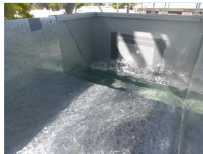
DB 500-1, Q = 16 l/s (box gutter slope - 1 in 200)
