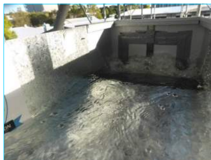
DB 300-1, Q = 16 l/s (box gutter slope - 1 in 200)
