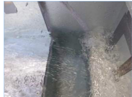
DB 300-1, Q = 16 l/s (box gutter slope - 1 in 200)
