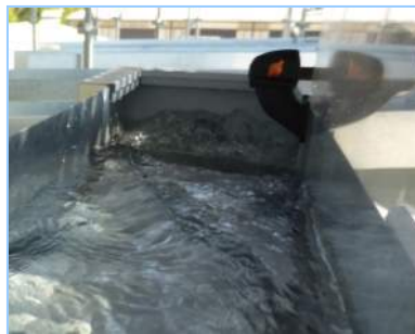
DB 200-1, Q = 16 l/s (box gutter slope - 1 in 200)
