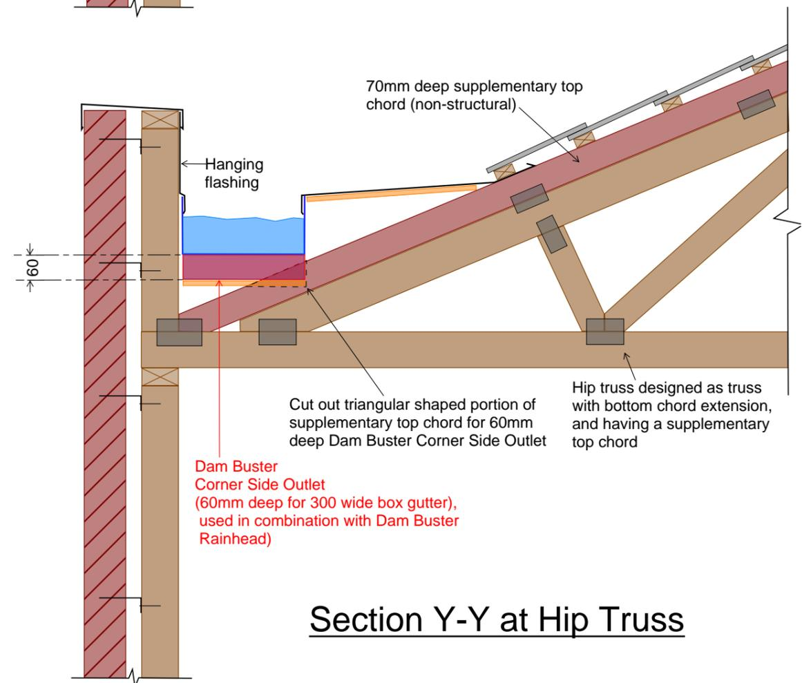
Section Y-Y at Hip Truss
