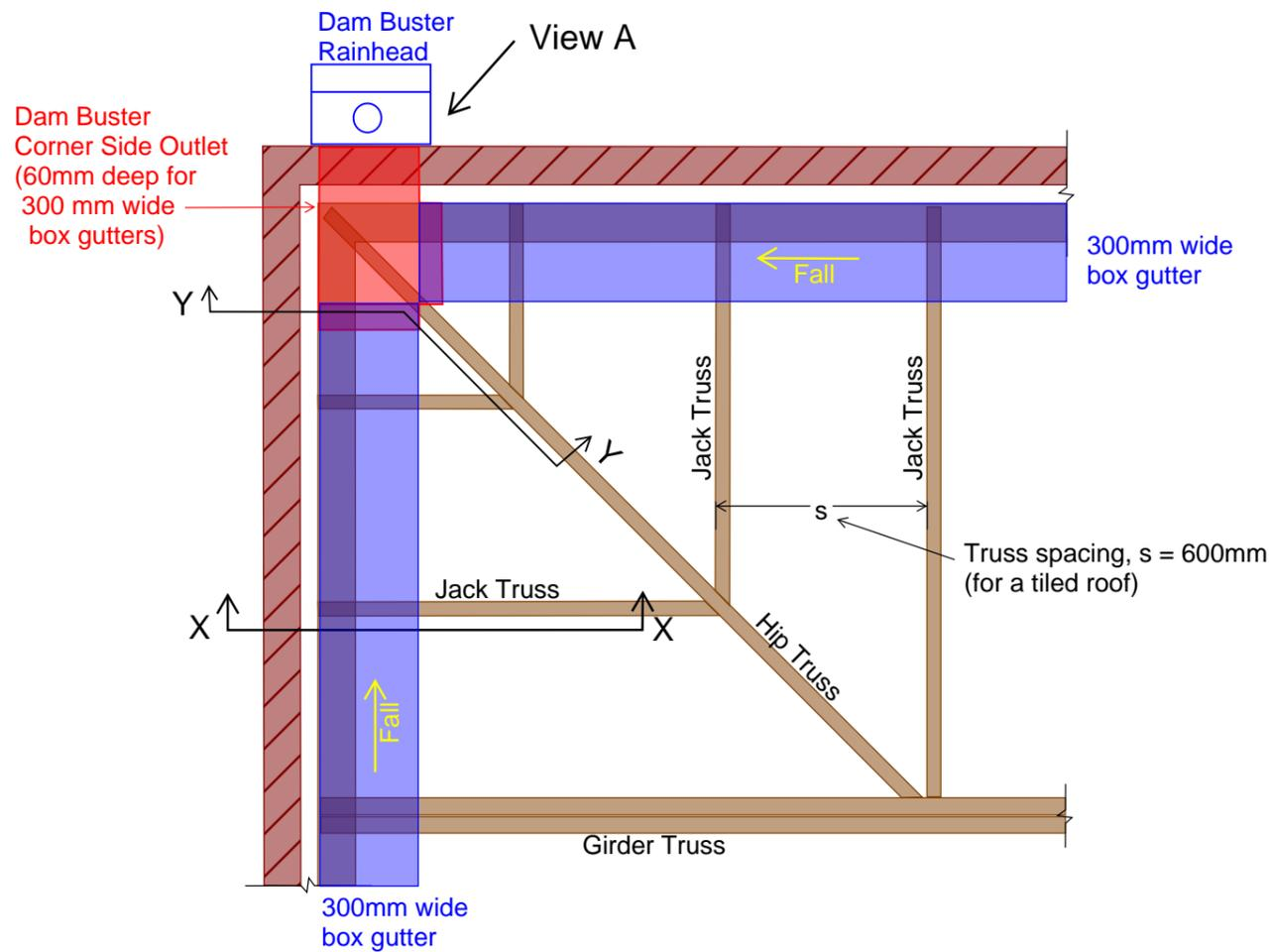
Plan at roof hip corner with parapet walls - Tiled roof
