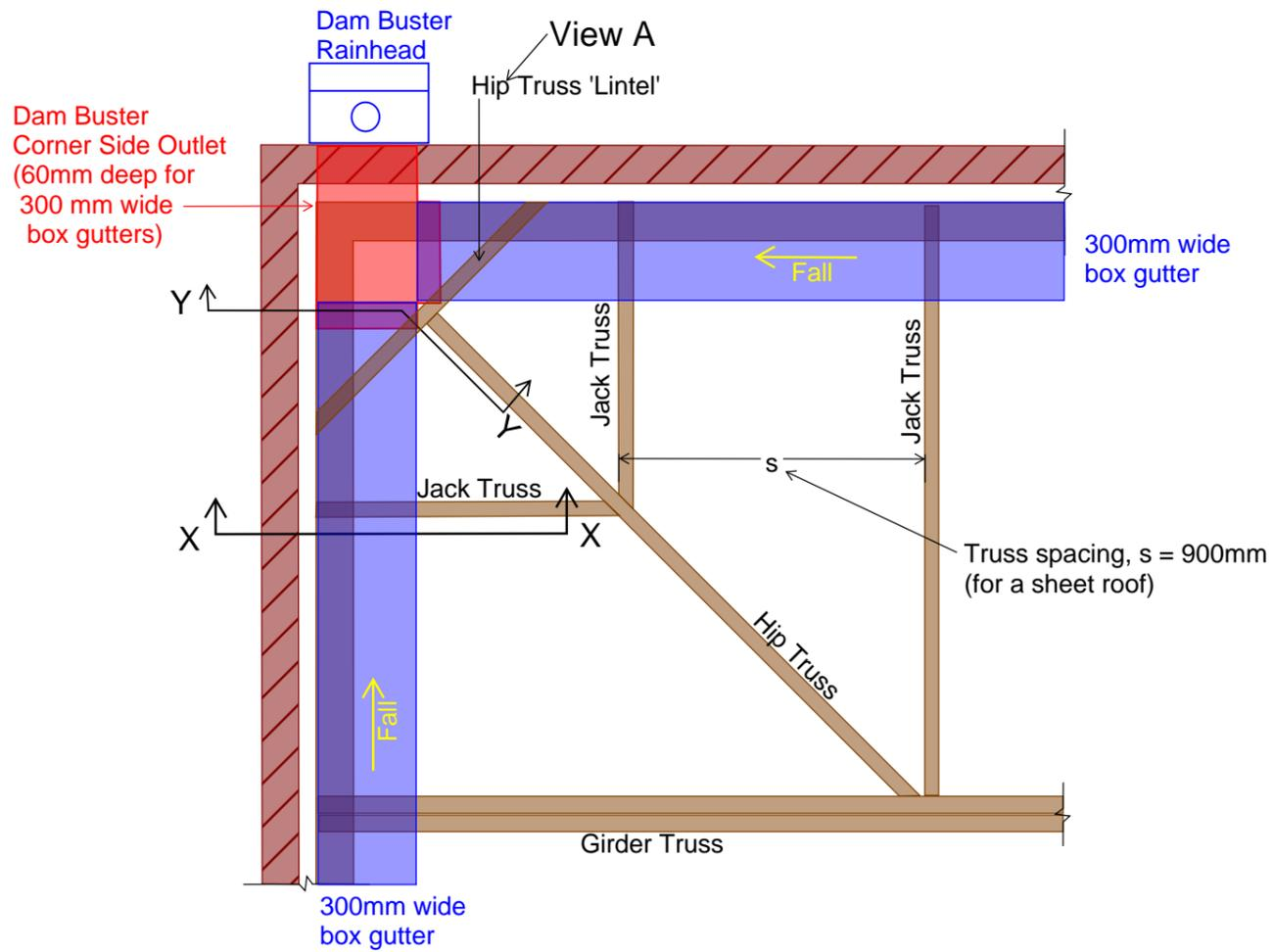
Plan at roof hip corner with parapet walls - Sheet roof
